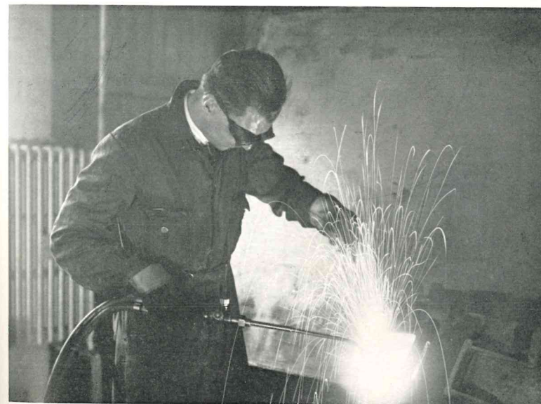
Thorne Workshop. Oxy-acetylene welder at work.
